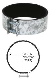
Manufactured from galvanized steel with an insulated rubber duct seal. These clamps facilitate the connection and disconnection of round ventilation ducts. All models incorporate internal hanging tabs for suspending the ducting / fan when horizontally mounted.
