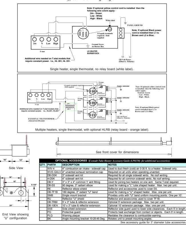
Typical Field Wiring Diagram
